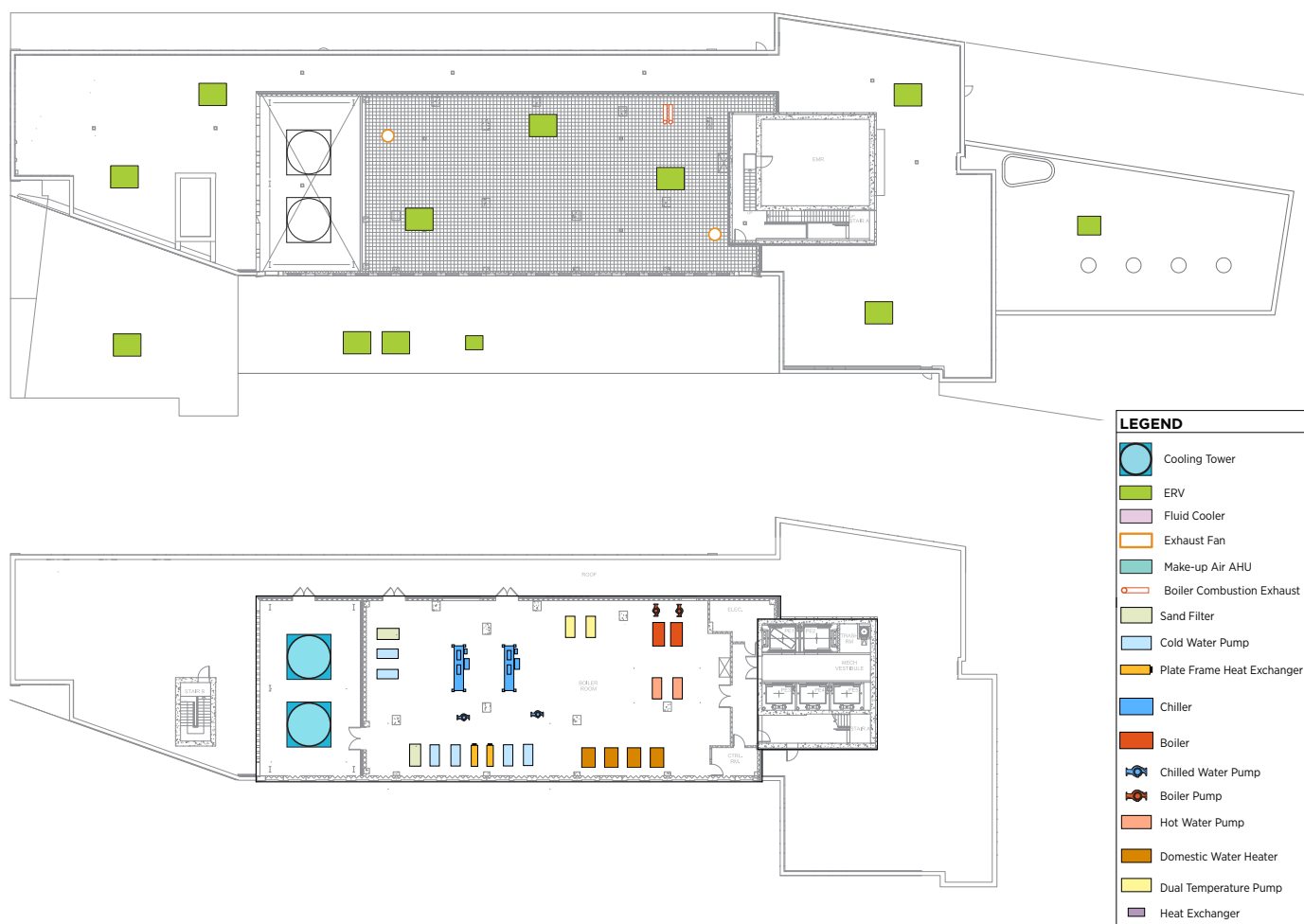
Figure 3.23b: Passivhaus Proposal - Composite roof plan (top) and Mechanical Mezzanine (below). Note: Two ERVs are not shown - one ERV serving the lobby is located in the package room, and one serving the commercial storage space is located in the ceiling of that room.
