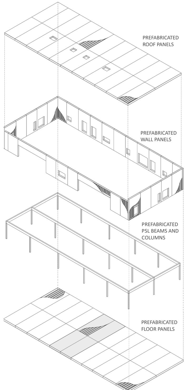
Gastown Childcare Centre axonometric drawing showing the prefabricated elements (Credit: Acton Ostry Architects)
