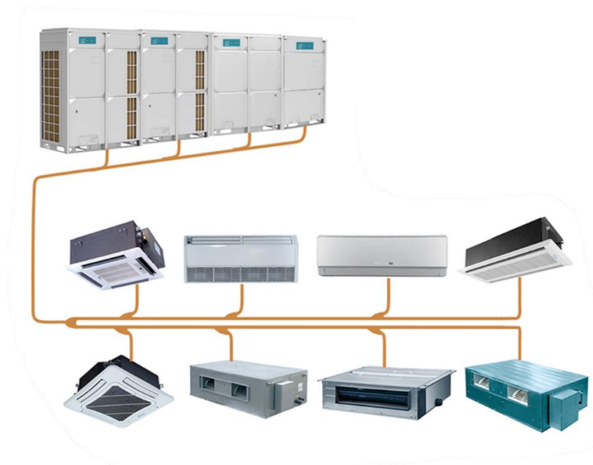
FIGURE 29: VRF SYSTEM SCHEMATIC
